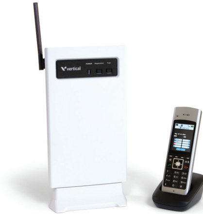
The Vertical V11000 Cordless DECT Phone set includes handset with charging stand and base power station, and supports up to six optional repeaters (sold separately).
